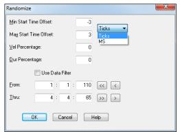
The **Min Start Time Offset** is the lowest amount of ticks that the program can move a note backward in time. The **Max Start Time Offset** is the highest amount of ticks that the program can move a note forward in time.
