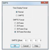
**Time Display Modes**: If the time display mode is set to Normal the time will be displayed in Measures:Beats:Ticks. When it is set to SMPTE, the time will be displayed as Hours:Minutes:Seconds:Frames.
