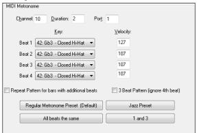
You can choose a different sound for each beat by using the Beat combo box to select a key from the list of drum notes for the standard GM drum kit. Use the Velocity setting to vary the volume of the notes in a rhythmic pattern.
