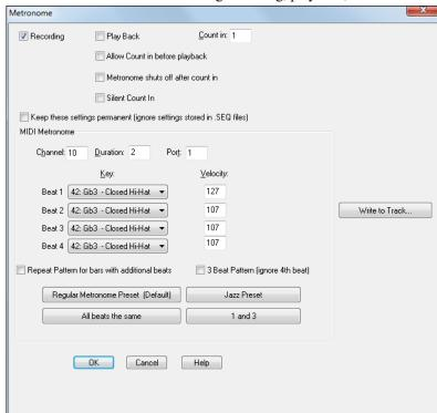
**Recording** - If this checkbox option is enabled the metronome will be **on/heard** during **recording**.
