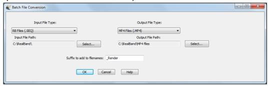
**Input File Type**: The Input File Type combo lists the most common MIDI and audio file formats plus RealBand and Band-in-a-Box file types. There is also the option to select "All Supported File Types" to convert a folder with more than one type of file.
