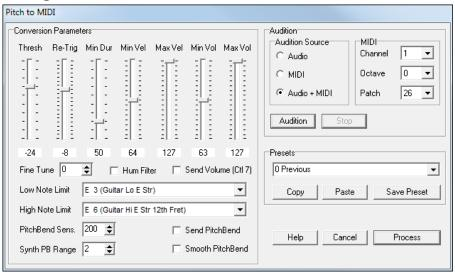
**Thresh** - The Note On level threshold, in dB. Audio below the Note On threshold will not trigger notes. If Thresh is set too low, the converter will try to convert noise and unintended notes to MIDI. If Thresh is set too high, the converter might miss some of the intentional notes in the audio.
