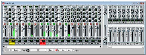
The Mixer track strips conveniently show the track name vertically to the left of the volume sliders. This is the track name that is assigned in the Tracks window, go to that window to add or change track strip names.
