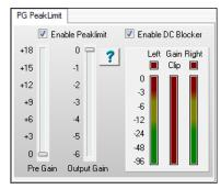
Audio Clipping happens when the audio is so loud that the sample numeric range is exceeded, and the tops of the waves are "clipped off."
