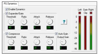
PG Dynamics will apply compression, expansion, or a combination of the two.
