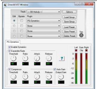
The [Load Group] and [Save Group] buttons let you load and save the effects settings for the currently selected track. The [Load Preset] and [Save Preset] buttons let you save and load presets for the current effect (such as Echo/Chorus). The [Delete Preset] button lets you remove a preset from the list of already saved presets.
