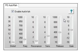
**Distort** adds some grit before filtering. When Distortion is set to a value of zero, there is no distortion. If attempting to AutoWah a mellow signal that doesn't have many high frequencies, you can crank the Distort slider to add some buzzy highs before filtering.
