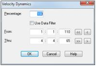
The **Percentage** setting will cause the velocity values to be moved either closer or farther away from the average velocity. A percentage setting of 100 results in no change. A percentage setting of 50 would compress the velocity values so that they are 50% closer to the average velocity. For example, if the average velocity is 64 and a note has a velocity of 84, the note's velocity will be moved midway between these values (64 and 84) to become 74.
