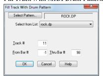
This feature is a convenient way of loading an existing drum pattern and pasting it onto a track. The [Select Pattern] button lists all of the available patterns in a drop-down combo so that you can quickly select a Drum Pattern file (\*.DP) to be pasted into the track that is selected in the "Track #" field.
