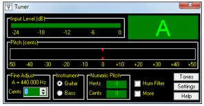
**Input Level:** Displays the instrument Input Level in dB. For best results, the level should peak at least halfway up. Quiet signals may be too noisy to properly recognize the pitch. Some inexpensive sound cards do not handle clipping gracefully. If your card seems to misbehave on very loud signals you should try to avoid hitting the very top of the level meter. On most sound cards, however, "going over the top" will not significantly affect the tuner's performance.
