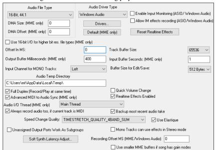
The **Audio File Type** combo box gives you a choice of sampling rates from 22.05K to 96K at bit depths of either 16-bits or 24-bits. 16-Bit, 44.1 is the file type to use for files that you want to burn to audio CDs.
