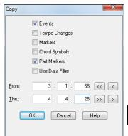
**Events Checkbox**: When this checkbox is enabled the Copy command will operate on MIDI events in the marked area of all selected tracks.
