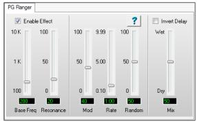
Interference between the original and delayed signals, makes a comb filter —many peaks and dips in the frequency response. As delay increases, more peaks and notches appear in the comb filter, and the frequency of the lowest peak/notch descends.
