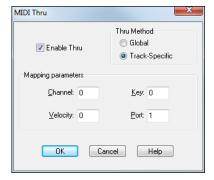
**Enable Thru**: If this option is checked the **MIDI Thru** feature will be enabled.
