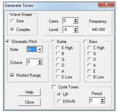
**Chromatic Pitch** - Select this radio button to select any desired note and octave.
