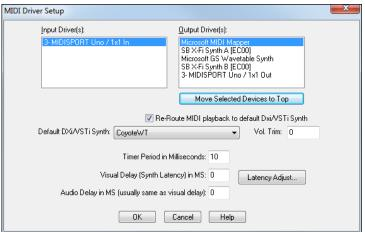
The [Move Selected Devices to Top] button lets you adjust the order of the MIDI Output ports. This means you can choose which MIDI Output devices appear as Port 1, Port 2, etc. within RealBand, rather than the default order for the ports determined by the operating system.
