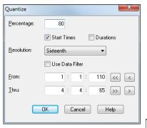
This is very useful for correcting timing errors in your music performance(s). Both the *start times* and *durations* of MIDI notes can be quantized. The *resolution* setting will determine the degree to which the timing is rounded. For example, if you choose a resolution of a sixteenth note, the notes in the marked area will be rounded off to the nearest sixteenth note. You may choose any resolution setting anywhere from a whole note down to a 32nd note.
