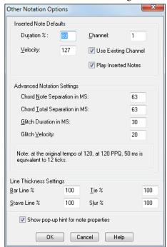
The **Duration %** setting causes the durations to be set to a percentage of the currently selected duration. For example, if the current duration is Whole, and you set the percentage to 50, the duration will be 50% of a Whole note.
