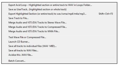
Export Acid Loop - Highlighted section or entire track to WAV in Loops Folder: This command will render the highlighted section of the current track or the whole track as an ACID Loop and save it to the bb\RealTracks\Loops folder.
